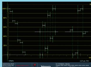
Figure A4: UHDTV1 YPbPr paraded waveform display with 100% color bar test signal, using BT.2020 colorimetry.
