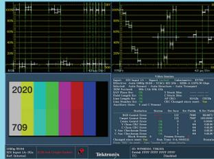
Figure A2: Using a 100% color bar signal to show conversion of RGB levels from 700 mv (100%) to 0mv (0%) for each color component with a color bar split field BT.2020 and BT.709 test signal. The WFM8300 was configured for BT.709 colorimetry as shown in the video session display.
