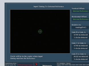
Figure C2: Input timing to external reference shown on the Tektronix WFM8000 Series Waveform Monitor.
