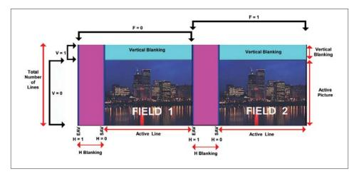
Figure 12. Layout of 2:1 interlaced digital frame.
