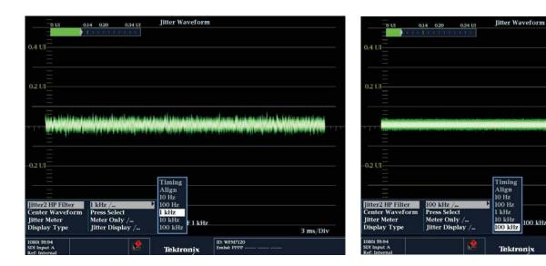
Jitter Display with 1 kHz Filter
