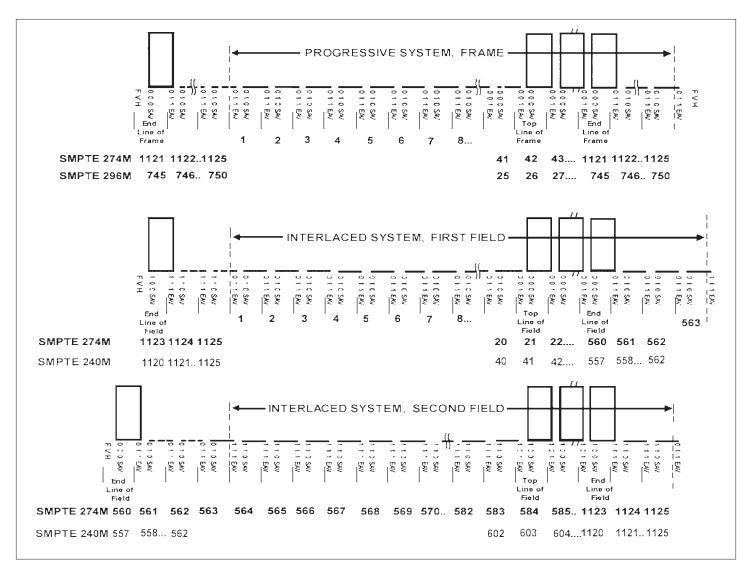
Figure 31. High-definition digital vertical timing.
