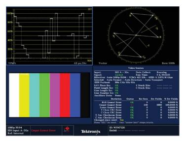
Figure 46. Fast progressive 1080p 59.94 3 Gb/s level A color bar signal shown on WFM7120.
