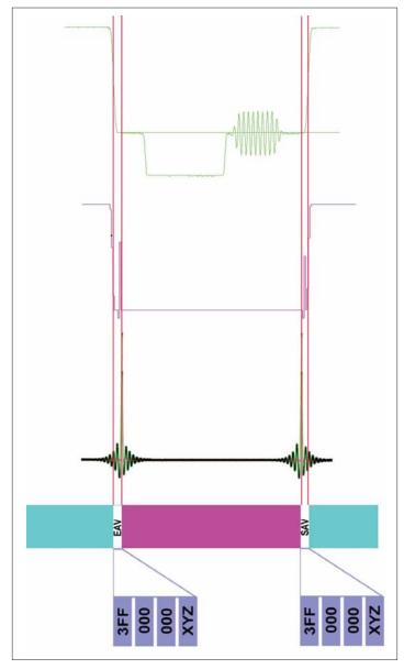
Figure 11. Digital horizontal blanking interval.
