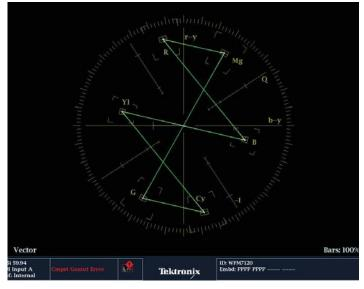
Figure 99. NTSC vectorscope display.
