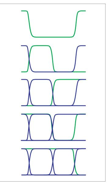
Figure 72. Development of the eye diagram.
