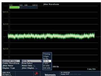
Jitter Display with 10 Hz Filter
