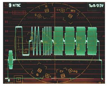
Figure 73. Multiburst test signal with equal amplitude at each frequency, 1H display.
