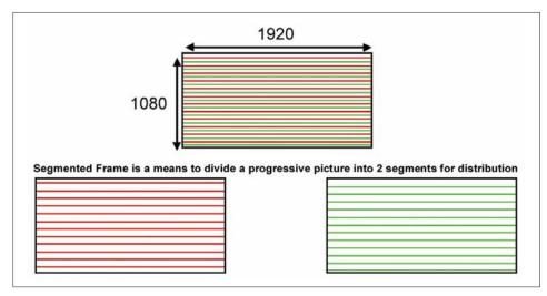
Figure 26. Conversion of a progressive frame into segments.
