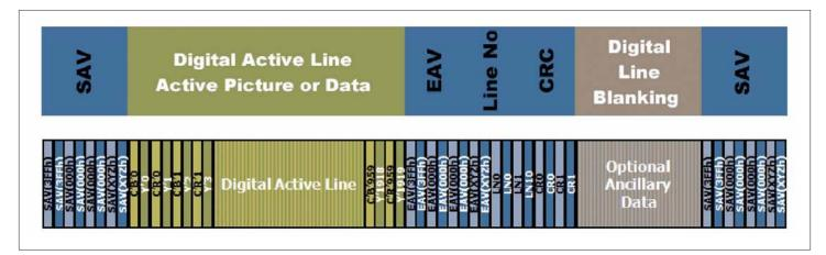
Figure 34. SDI data structure for a single line.
