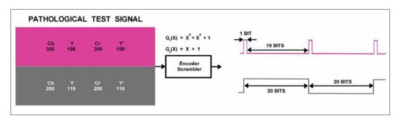
Figure 78. SDI Check Field "Pathological Test Signal."
