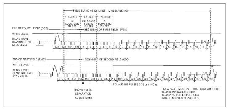
Figure 23. PAL vertical blanking interval.
