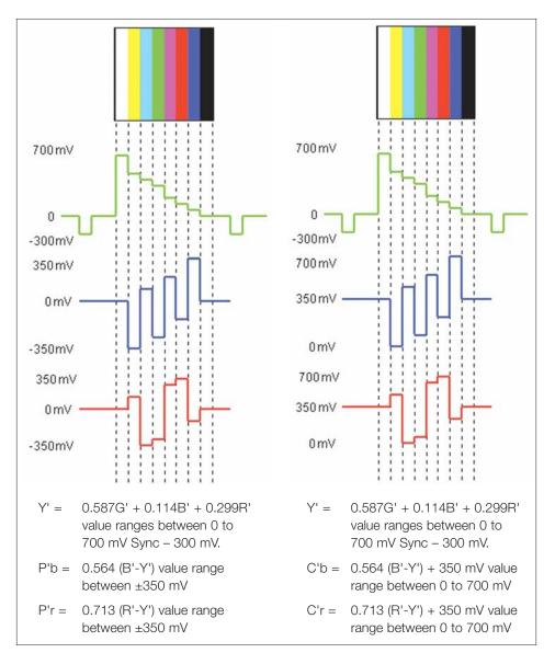
a color-difference set will produce subtle changes in hue or changes in saturation only. A low level in R'G'B', however, will produce a distinctly wrong-colored image. The concept of transcoding R'G'B' to one luma and two colordifference signals has proven very useful. Such signals, with relatively minor variations, are the basis for all existing component video formats and also for composite broadcast standards throughout the world.
