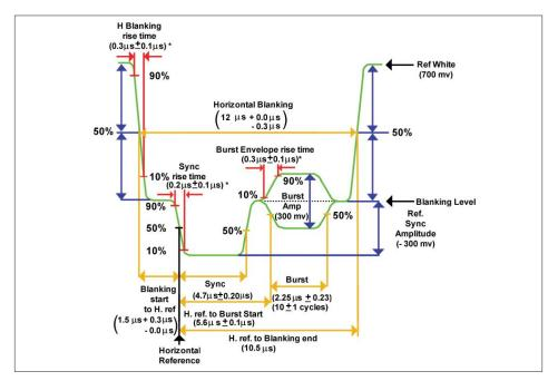
Figure 19. PAL horizontal blanking interval.
