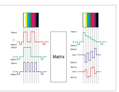
Figure A4. Matrix of R'G'B' signal-to-color difference.
