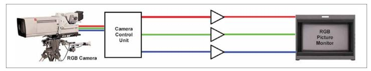
Figure 1. RGB from the camera with direct connections to the monitor.
