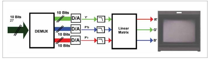
Figure 8. Recovering analog R'G'B' from parallel data.
