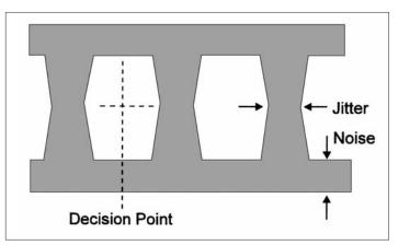
Figure 82. Data recovery of serial signal.
