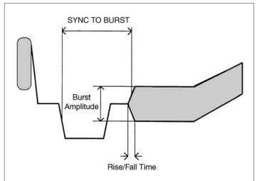
Figure C2. SECAM system horizontal interval.
