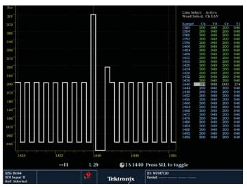
Figure 28. 270 Mb/s EAV timing reference packet viewed as an analog luma channel signal.
