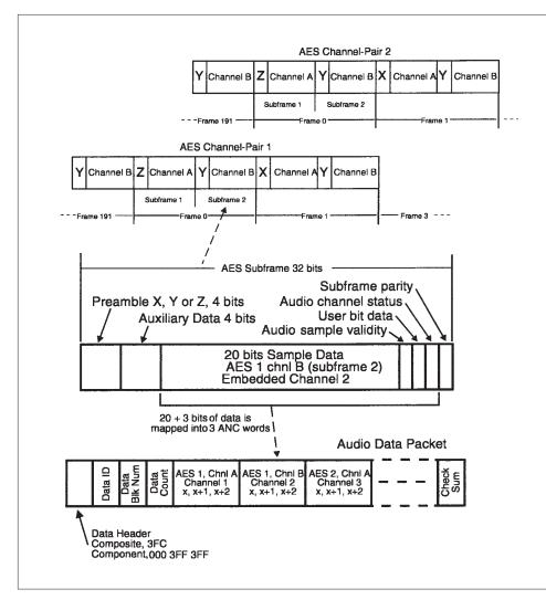
Figure 54. Basic embedded audio.
