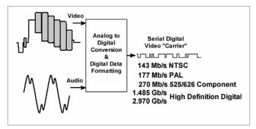
Figure 13. The carrier concept.
