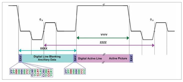
Figure 16. Ancillary data in the digital line vs. analog representation.
