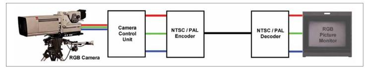
Figure 2. Video encoded to NTSC or PAL for transmission on a single coaxial cable.
