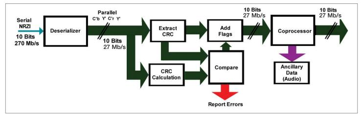
Figure 7. SDI Receiver - deserializes the video data to parallel.
