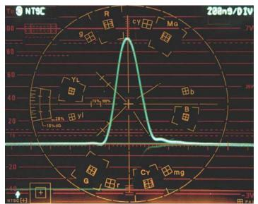
Figure 76. 2T pulse and bar, degraded.
