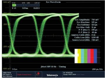
Figure 84. Non-symmetrical eye display on WFM7120.
