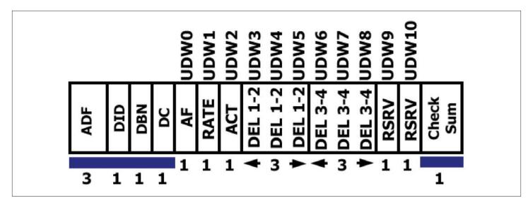
Figure 58. Structure of audio control packet.
