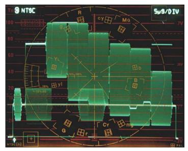
Figure 70. Correctly adjusted composite video amplitude, NTSC, no setup.
