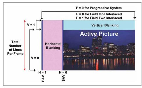
Figure 17. Spatial layout of the digital frame with V, F, and H-bit values.
