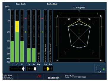
Figure 62. Surround Sound Display with live audio signal.
