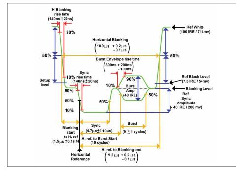
Figure 18. NTSC horizontal blanking interval.
