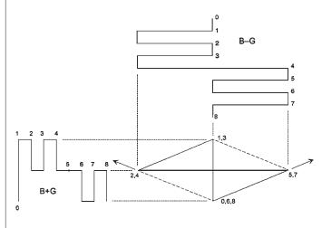
Figure 106. Development of the Diamond display, upper half.
