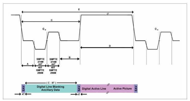
Figure 20. High-definition line timing.
