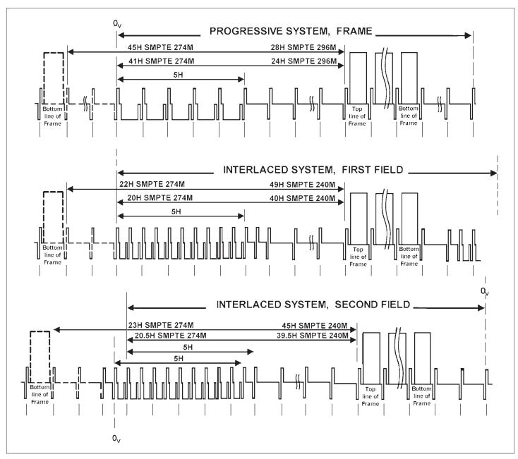
Figure 24. Analog high-definition vertical blanking interval.
