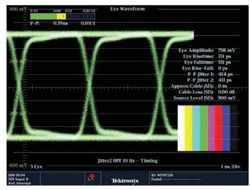
Figure 71. Correct 270 Mb/s data signal viewed with WFM7120.
