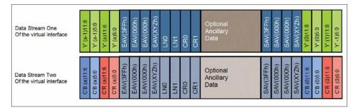
Figure 52. Level A Y'C'bC'r mapping structure four.
