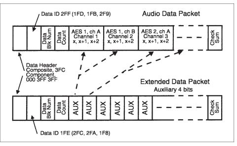
Figure 55. Extended embedded audio.
