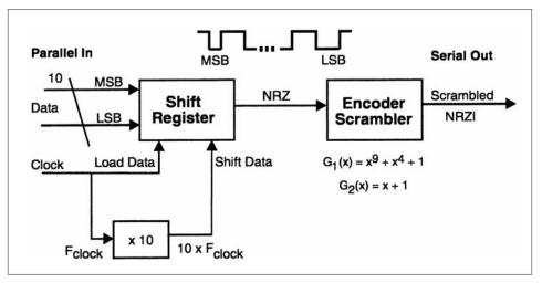
Figure 14. Parallel-to-serial conversion.
