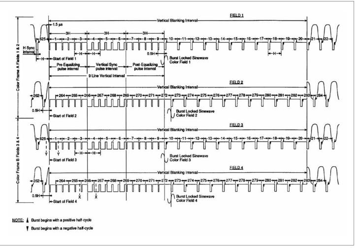
Figure 22. NTSC vertical blanking interval.
