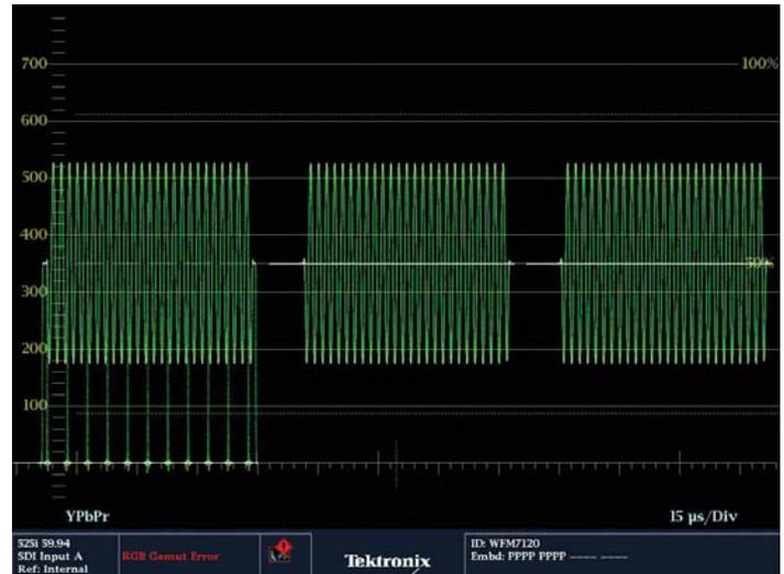
Figure 93. Bowtie test signal.
