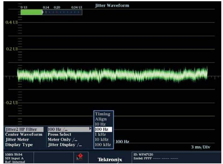
Jitter Display with 100 Hz Filter
