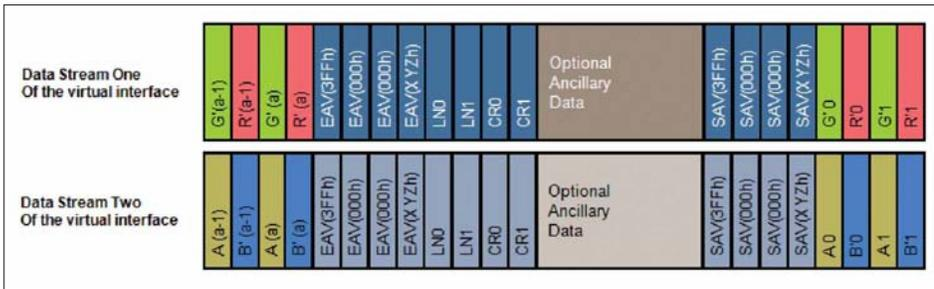
Figure 50. (Level A) R'G'B' mapping structure two.
