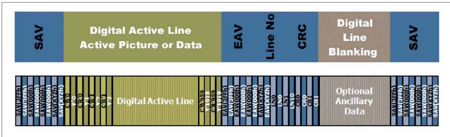
Figure 34. SDI data structure for a single line.
