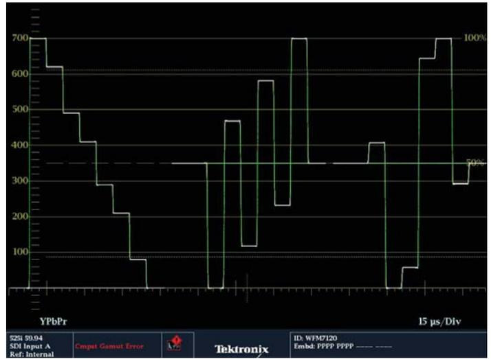
Figure 98. WFM7120 Y/C'b/C'r display of 100% color bars.
