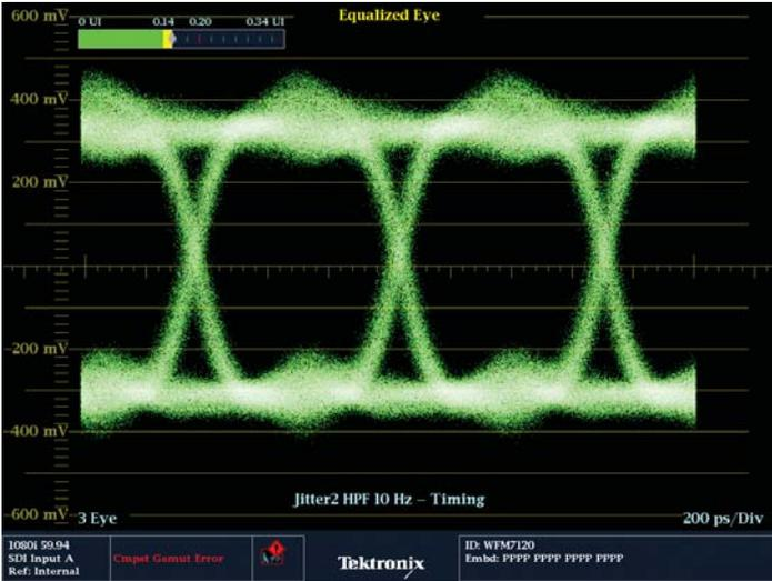
Figure 83. Underterminated Eye display on the WFM7120.
