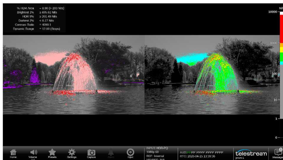
Tektronix display showing false color mode to show out of gamut colors.
