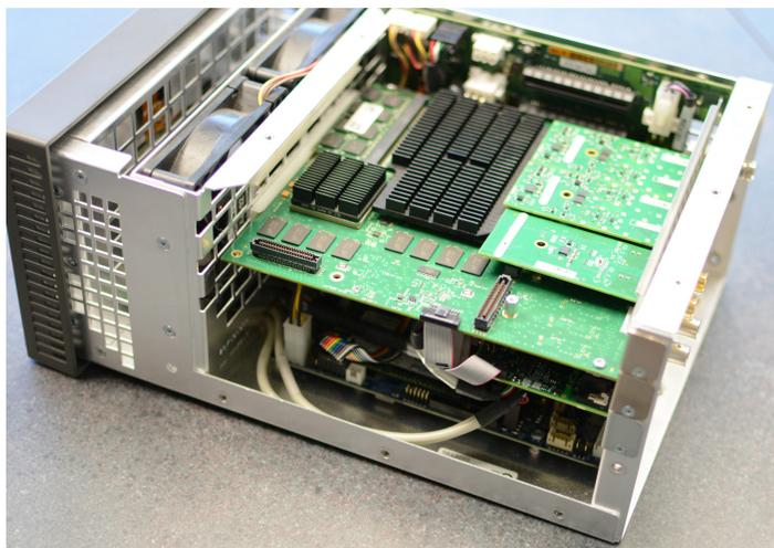
Figure 4: Mezzanine board removed
