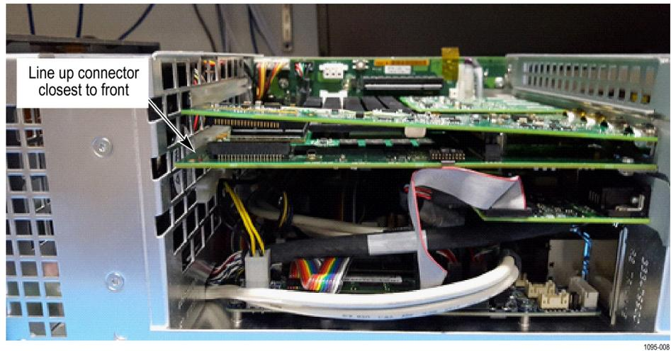
Figure 8: Line up the front connector
