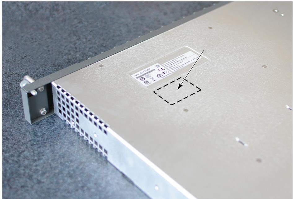
**Figure 28: Installing the MPX-UP serial number label**
