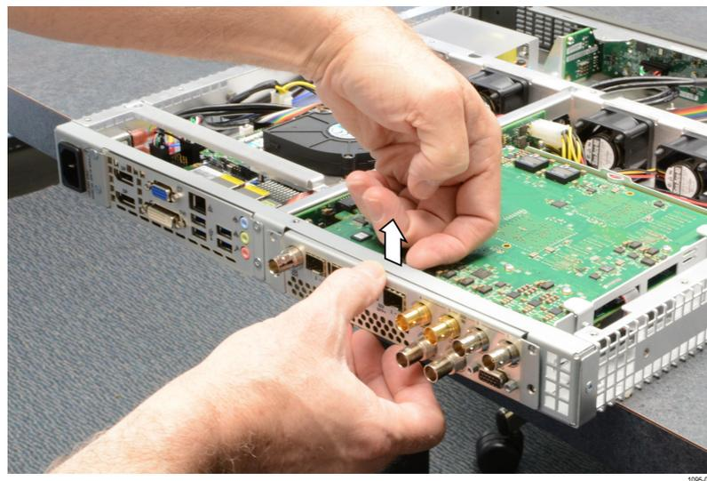
**Figure 27: Install the rear plate panel**
