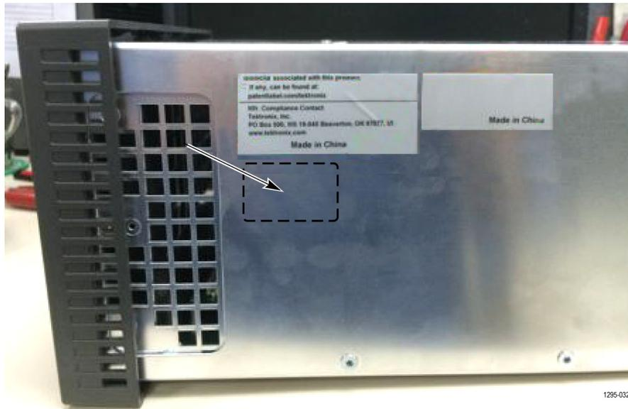
Figure 11: Installing the MPI-UP serial number label
