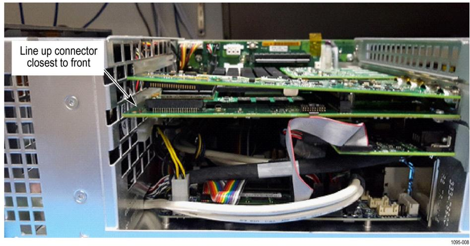
Figure 8: Line up the front connector
