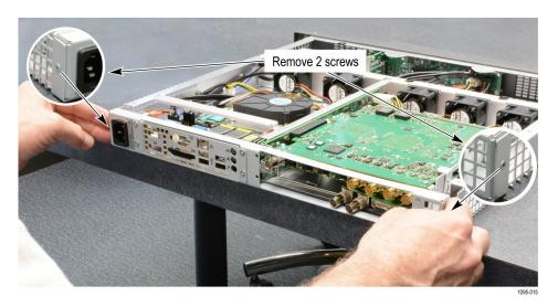
Figure 16: Remove the back panel
