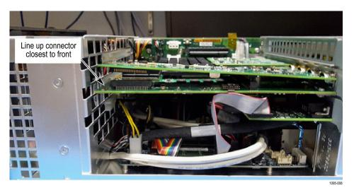
Figure 8: Line up the front connector
