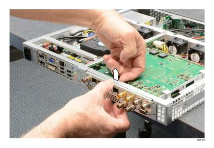
Figure 27: Install the rear plate panel
