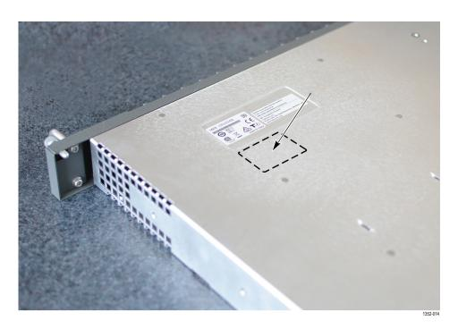
Figure 28: Installing the MPX-UP serial number label
