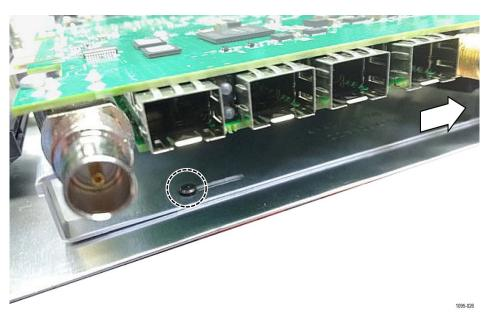
Figure 25: Slide the Mixed Media module back into chassis
