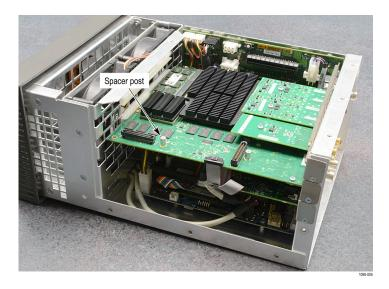
Figure 5: Spacer post installed
