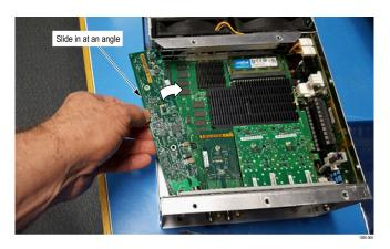
Figure 6: Eye mezzanine board placement
