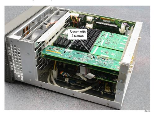
Figure 10: Finish the 12G Eye mezzanine board installation
