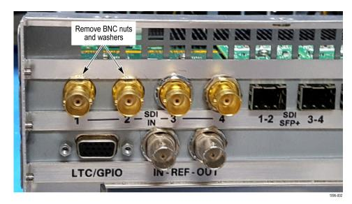
Figure 2: Remove the BNC nuts and lock washers
