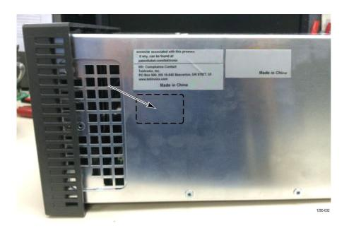
Figure 11: Installing the MPI-UP serial number label
