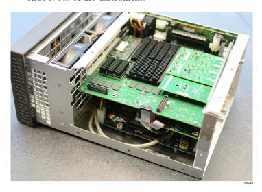
Figure 4: Mezzanine board removed
