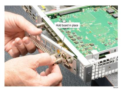
Figure 26: Secure the GPIO board on the rear plate panel
