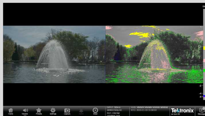
Figure 3: Using banded False Color is an easy way to help set exposure levels.
