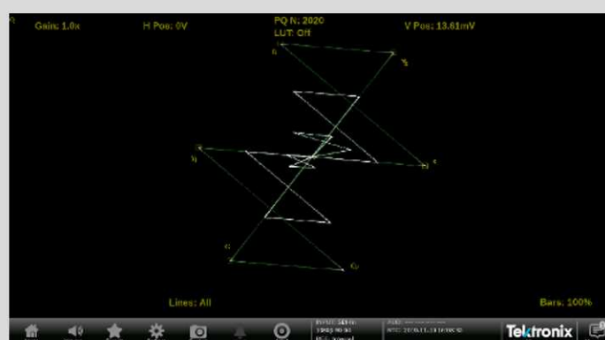
Figure 5: Vectorscope displays – top is for a Rec. 709 and bottom shows the impact of Rec. 2020 (for color bar input).
