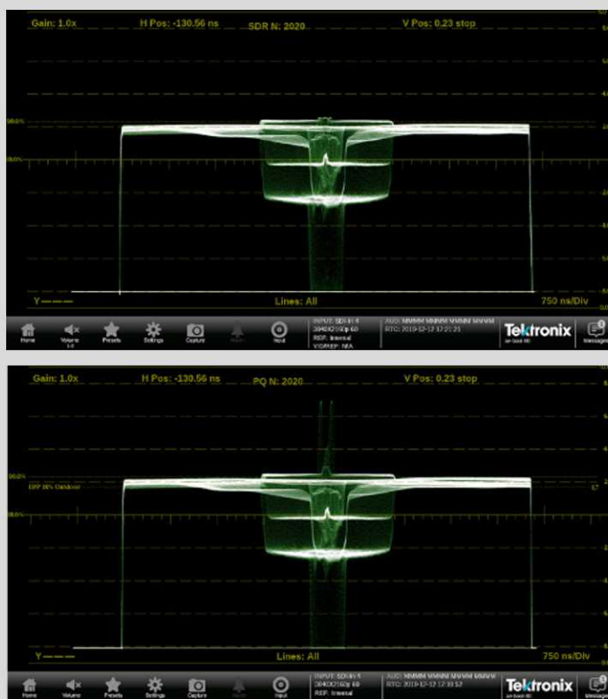
Figure 2: Shows the same SDR and HDR signals as in figure 1, but in this case, they are displayed in a STOP display with levels being set by light or luminance levels. Comparison is easier because both images look very similar, the light levels can be compared. The key difference is that the specular highlights are shown on the HDR waveform, but are cropped (as expected) on the SDR waveform.
