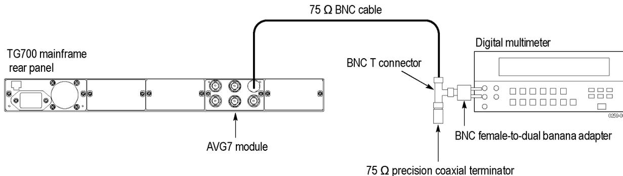
2. On the TG700, press the **MODULE**, **FORMAT**, and **FRONT PANEL ENABLE** buttons simultaneously, and then release the **MODULE** and **FORMAT** buttons to restart the instrument in Factory mode. Continue holding down the FRONT PANEL ENABLE button until the “TG700 start up with Factory Mode” message appears. Allow the TG700 to load and configure; it is finished when TG700:PRESET message appears.
