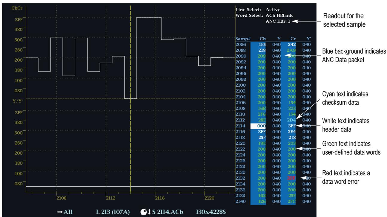
Figure 6: Datalist display showing ANC Data packet highlighting
