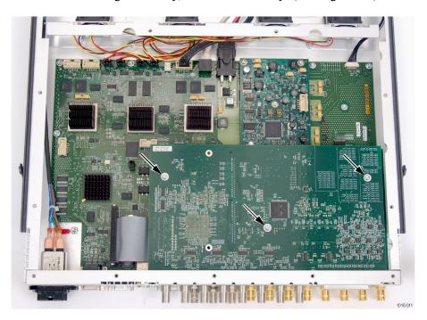
Figure 14: Audio board screws
