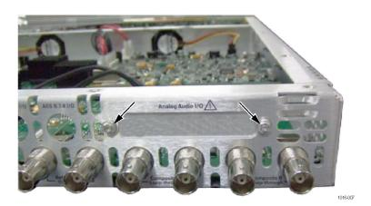
Figure 12: Remove blank cover for audio connector
