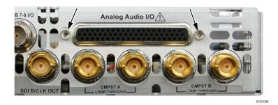
Figure 15: Audio connector retainer posts
