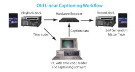
Traditional legacy captioning gear required expensive and complicated setup, worked only with tape, and caused generation loss in video quality.
