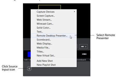
To create a new Remote Desktop Presenter shot, select *New* and enter a source name (shot name). Enter a Source Name, an IP Address of the remote computer, and (optionally) check Enable Audio if the want the audio from the remote computer to be included. Click OK when finished.
