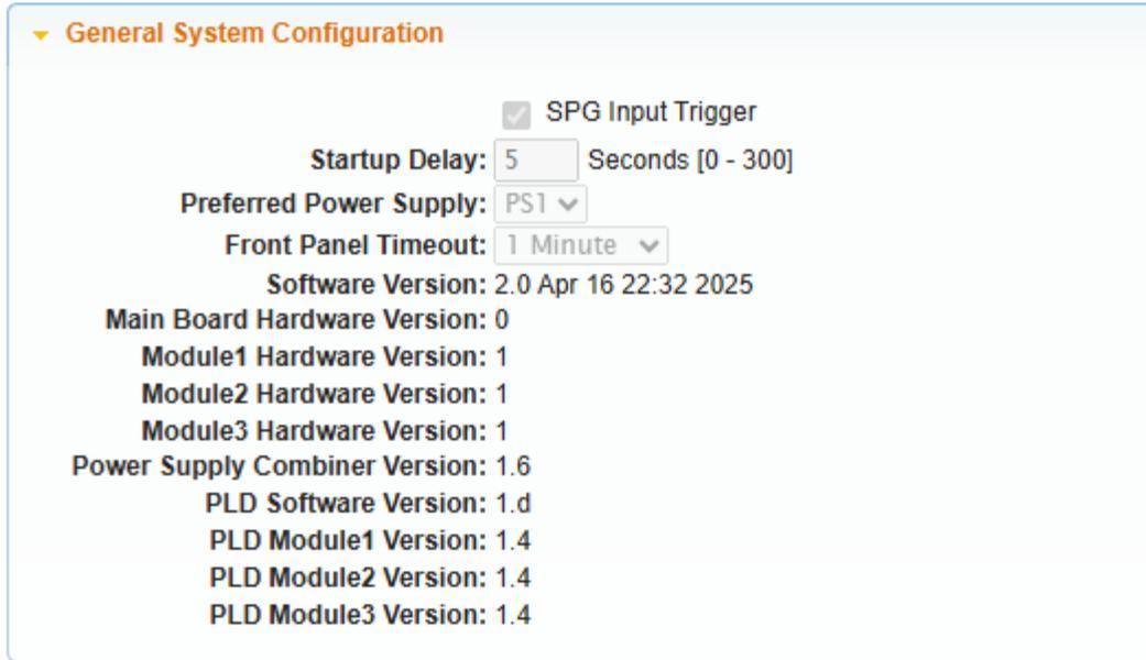
On the front-panel interface, go to the **SYSTEM CONFIG** menu and press **ENTER**. Press the up or down arrow buttons to navigate to the **FW VERSION** submenu. Press the left or right arrow button to see both the version number and date.
