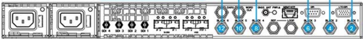
Channels 7–9 on the ECO8000 should be used for any of the SDI 1–4 outputs from the SPG9000. These three channels could also be used for WORD CLK and/or DARS outputs from the SPG9000 if 5 or 6 BLACK outputs are being used.
