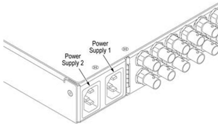
The front panel has two LED indicators for each power supply. The upper LED (labeled “AC”) refers to the state of the external mains connection and the lower LED (labeled “DC”) refers to the state of the power supply module. See [Power Supply Status](#) for complete descriptions of these indicators.
