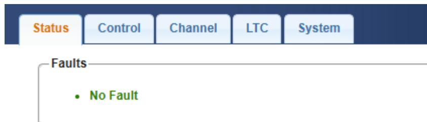
If there are any active faults, the Status tab name will be colored red and an error indicator will be displayed, so if any other tab is currently open, you will see the fault notification. Additionally, the browser tab will display the red indicator and "ALERT" is added to the tab name, so if any other browser tab is open, you can be alerted to the ECO8000 fault.
