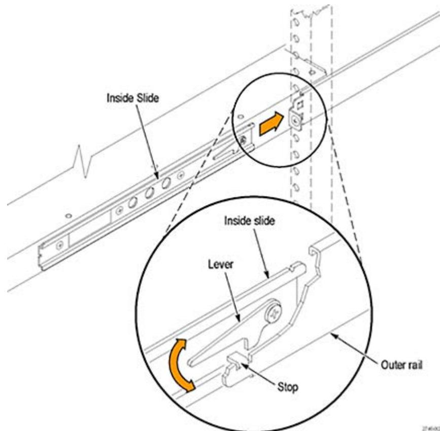
2. Push the instrument into the rack until it stops.
