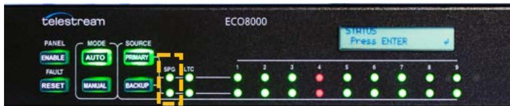
To configure the SPG input trigger from the front panel, go to the top-level **SYSTEM CONFIG** menu and press **ENTER**. Press the up or down arrow buttons to navigate to the **SPG INPUT TRIGGER** submenu.
