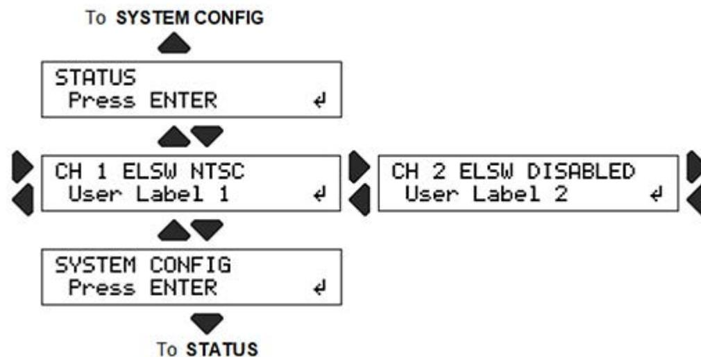
Submenus in the nested hierarchy are indicated by one or more arrow indicators preceding the menu name on the top line of the display. Press the **BACK** button to return to the previous level.
