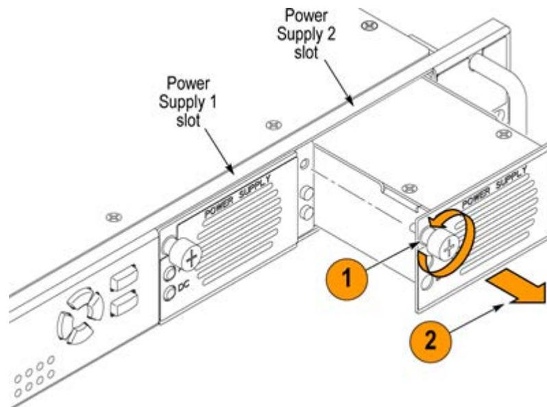
Insert the replacement supply module into the instrument until it latches into place and then turn the retaining screw clockwise to secure the module in the chassis.
