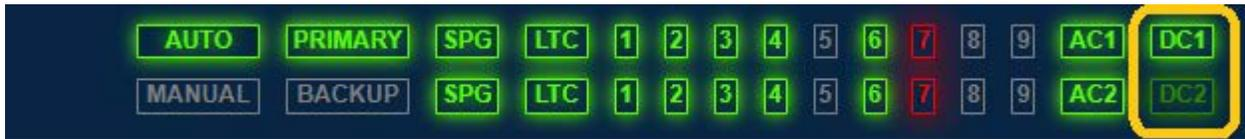
The recommended usage strategy is to configure one supply as preferred and use the second supply only in case the first supply has a failure. This usage strategy allows the backup supply to have the maximum remaining life when it is needed.
