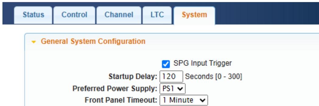
On the front-panel interface, return to the top menu, go to the **SYSTEM CONFIG** menu, and press **ENTER**. Press the up or down arrow buttons to navigate to the **PREFERRED SUPPLY** submenu and press **ENTER**. Select **PS1** or **PS2**.
