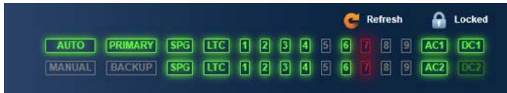
The top row of 11 LEDs show the status of the signals from the Primary SPG9000 source and the bottom row shows the status of the signals from the Backup SPG9000 source.
