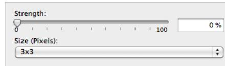
**Strength (%).** use the slider (or manually enter the value) to set the amount of smoothing to apply. Range: 0 to 100. Higher values provide stronger smoothing.
