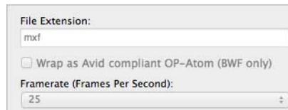
**Wrap as Avid compliant OpAtom (BWF only).** Check to generate a file using the proprietary modifications to the standard for Avid video editing systems.
