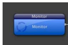
A monitor source polls a specific computer and directory at regular (user-settable) intervals. When a file is saved in the target directory, it is identified and a job is scheduled for encoding. However, writing the entire media file to the directory takes time and the file cannot be encoded until the file transfer is complete, so the monitor polls the file to see when the file is completely written and released. Only then is the encoding job submitted.
