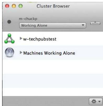
A cluster is a named collection of computers with Episode installed that work together to process Episode workflows. Each instance of Episode running on a computer is called a node. You can define a cluster temporarily to process a specific large job, or you can create clusters and leave them in operation for long periods.
