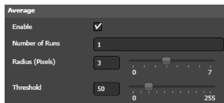
Figure 169. Noise Reduction Filter Settings—Average Method
