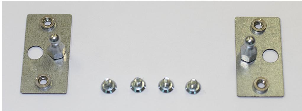
2. Remove the old two chassis rack ear brackets and four retaining screws from the chassis.
