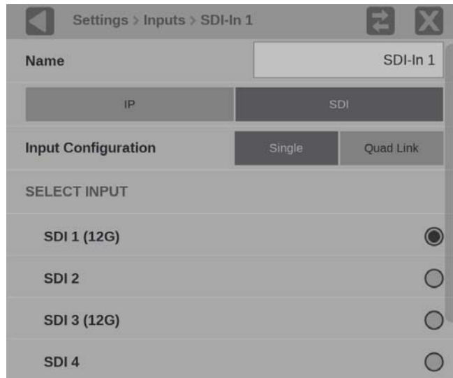
Figure 33: Quad Link SDI signal configuration
