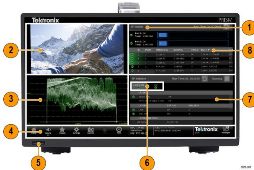
Figure 6: Elements of the front panel
