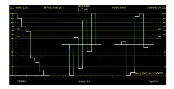
10. Set 3D LUT: Convert to Rec. 709 to On to allow trace displays to convert the Gamma and Color Gamut settings for the signal to SDR Narrow and BT. 709 or use a custom Favorite LUT.
