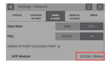
o If the SFP module speed does not match the Data Rate setting, instead of the data rate and frequency, the message "SFP not compatible with selected Data Rate" appears.
