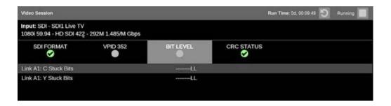
Y Stuck Bits: Displays which of the luminance video bits are stuck. If the readout is "---", then none of the bits are stuck.
