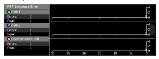
In the Reconstructed Path Errors section, 0 means no sequence errors have been detected, and any number (not 0) means sequence error or errors were detected after RTP packet reordering on each path and ST 2022-7 seamless reconstruction process.
