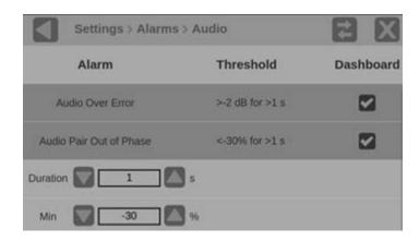
The percentage describes the location on the correlation meter (below the Lissajous image) in the Audio application. So long as the phase marker (green diamond) does not drop below -30% (in the example setting) for more than a second, the alarm will not occur.
