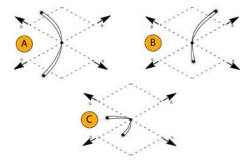
**Note:** Bending of the transitions indicates timing delays. When a color bar signal is applied, the vertical axis becomes an indicator of delay errors. Monochrome signals appear as vertical lines. Nonlinear component processing, such as from a gamma corrector that alters white balance, can cause deviations along the vertical axis.
