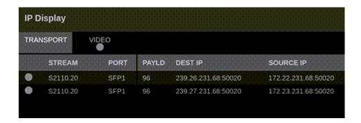
If you have an IP Generator license, you can check the receiver device and signal path via the IP Generator application, which provides ST 2110 -20/-30 with ST 2022-7 test signals.
