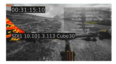
♦ Original Color: This mode Indicates the color(s) that exceed the Rec. 709 and P3 gamut limits for signals using the Rec. 2020 color gamut. This mode indicates colors that need correction. The colors indicated are out of gamut.
