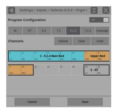
♦ 7.1.4 is immersive audio and requires 12 channels: eight for the audio main bed, or level-marked in cyan, and four for the audio upper bed, marked in orange.
