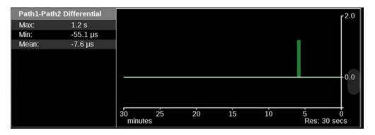
**Note:** The measurement range of Path1-Path2 differential measurement is 1 second.
