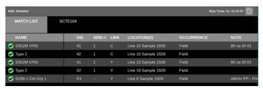
**Note:** A green checkmark in the WATCH LIST name column means data is being continuously received. A yellow exclamation mark means data has been received but it has stopped.
