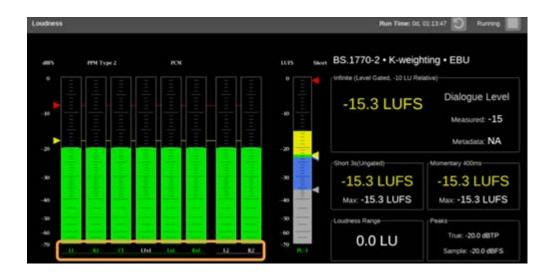
**Note:** The low-frequency effects channel (Lfe1) in 5.1 and 7.1 is not used in the loudness calculations.
