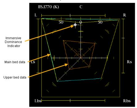
**Note:** In the Analyzer Layer, the Both layer is selected, but there is no upper bed data, as in non-immersive surround programs like 5.1, or 7.1, the upper bed surround display is empty (no orange display) because there is no upper bed audio data.
