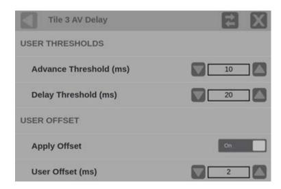
**4.** The Advance Threshold number is the time the audio test signal can arrive before the visual test signal arrives (to the left of the 0 line) and not register as an error; that is, the channel is green in the display. To change the Advance Threshold number, in the **Advance Threshold** box, type the number or select the up or down arrows.
