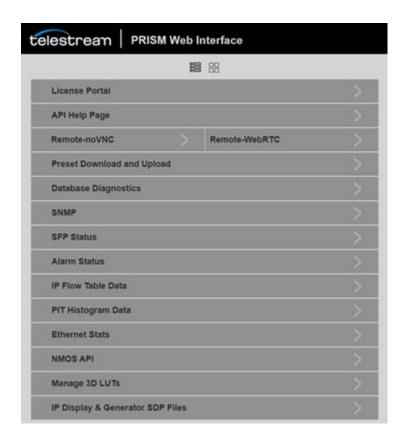
2. In the IP Display SDP File(s) section, select Display1 SDP File or Display2 SDP File to view the contents of the file
