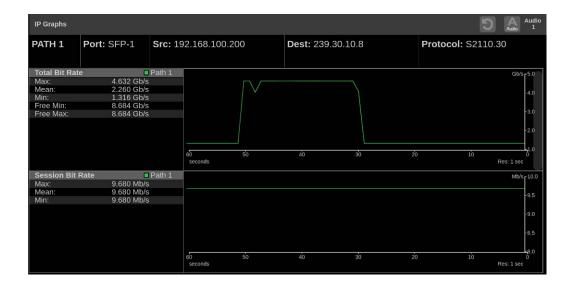
If ST 2022-7 monitoring is configured, the IP Graphs application includes Path 1 and Path 2. The graph data can be switched between viewing only Path 1, only Path 2, or both by selecting the Path button in the upper right of the screen.
