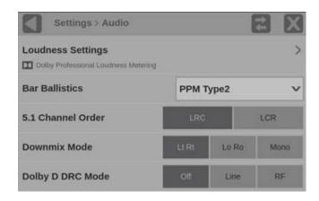
**5.** Select the **Downmix Dynamic Rng.: Line** or **RF**. These DRC compression factors are applied when downmixing to the various Dolby D listening modes.
