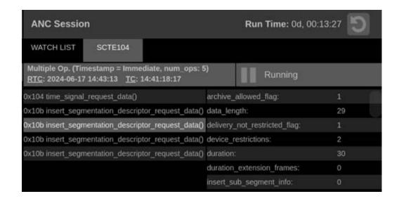
Note: The RTC (real-time clock) and TC (time code) numbers on the SCTE104 page match the RTC and TC in the PRISM status menu.
