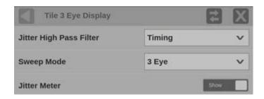
4. From the Jitter High Pass Filter list, select the high pass filter: Timing, Align, 10 Hz, 100 Hz, 1 kHz, 10 kHz, or 100 kHz.
