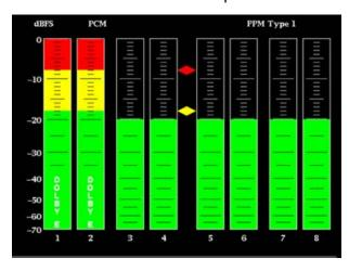
• The meter bars are displayed below the Test level in green.
