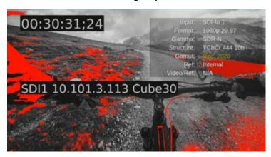
◆ Banded Color: This measurement is applicable only for signals that use the Rec. 2020 color gamut. Banded color indicates pixels that exceed the Rec. 709 or P3 gamut limits as contained in the Rec.2020 color gamut.
