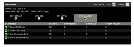
Note: The instrument uses the RP 165 standard for error checking. For HD and 3 Gb/s signals, the CRCs change on every video line.
