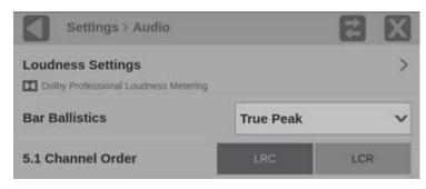
C. In the 5.1 Channel Order section, select LCR or LRC. The level meter reorders to left-center-right or left-right-center.
