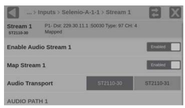
Note: ST 2110-30 or ST 2110-31 can carry PCM or Dolby D, D Plus, or Dolby E, but if ST 2110-30 will carry Dolby content, the data must be transmitted in pairs and set to start on odd channels such as 1-2 or 3-4.
