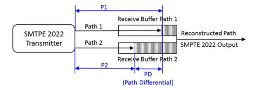
The ST 2022-7 specification defines Path Differential as an absolute value, but the Path1-Path2 Differential graph shows the signed value of Path 1 minus Path 2. A positive value means that Path 2 is lagging Path 1. The ST 2022-7 specification defines Path Differential as an absolute value, but the Path1-Path2 Differential graph shows the signed value of Path 1 minus Path 2. A positive value means that Path 2 is lagging behind Path 1.
