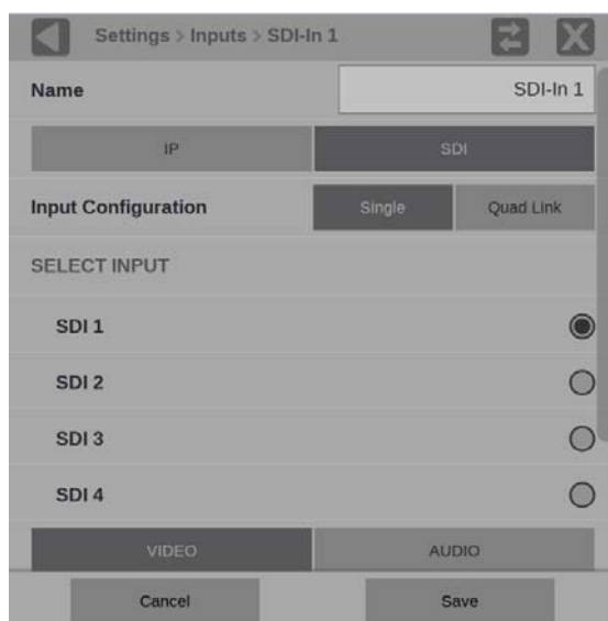
Figure 22: Single SDI signal configuration, SDI 1 input selected
