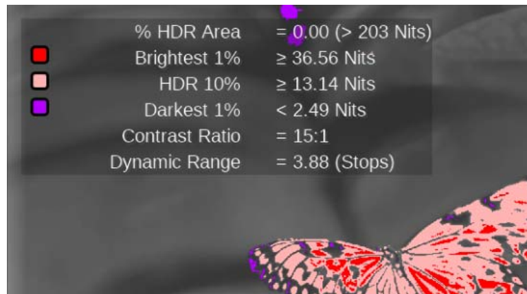
Figure 122: False Color display with Picture Measurements Overlay
