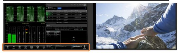
Figure 9: Extended display with the Status bar, on the primary screen, marked
