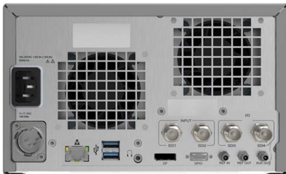
Labeled PRISM MPS-100 Rear-Panel Connectors
