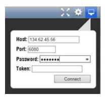
The web browser connects to the instrument with the browser display appearing exactly like the display on the external monitor.
