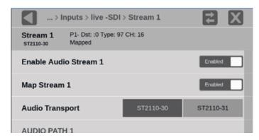
**Note:** 2110-30 or 2110-31can carry PCM or Dolby D, D Plus, or Dolby E, but if 2110-30 will carry Dolby content, the data must be transmitted in pairs and set to start on odd channels such as 1-2 or 3-4.
