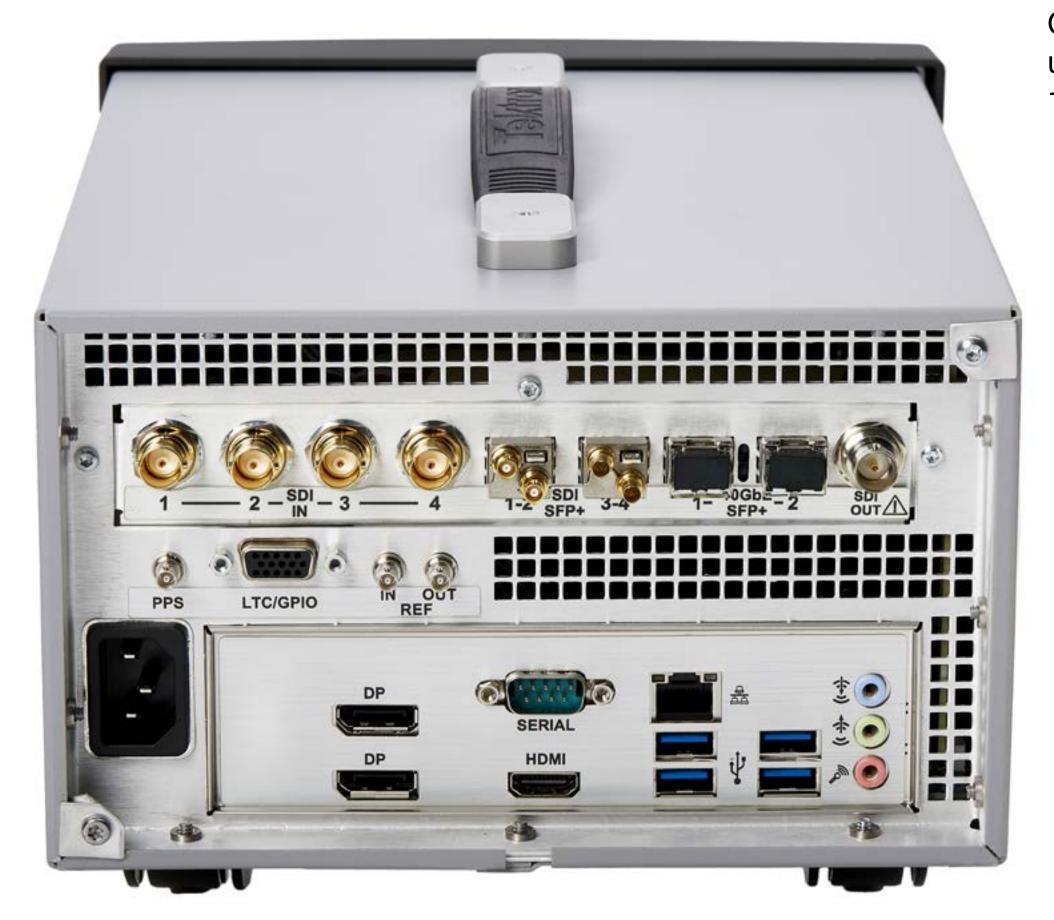
On the MPI series the 10G Mixed Media Card (MMC) can be identified by standard BNC used for SDI inputs and outputs along with multiple SFP+ cages for SDI outputs and 10GE IP Media ports. The reference BNCs are different between MPI and MPI2 models.
