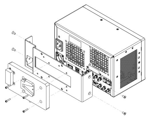
**6.** Set the MPS upright and remove the cover.
