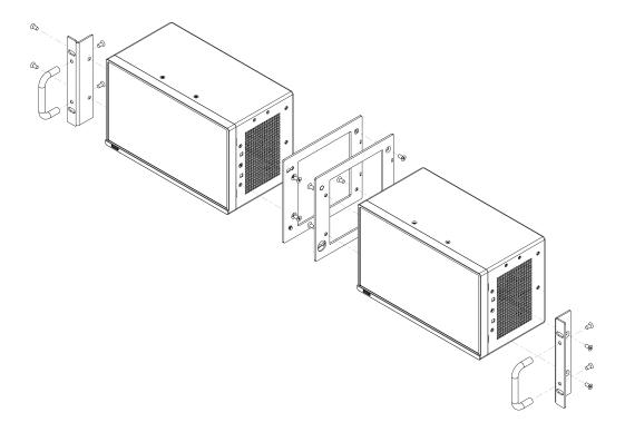
3. Insert the MPS assembly into the rack and align the rack-ear brackets at the correct level.
