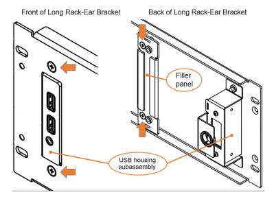
2. Choose which side of the rack the MPS will be on, set the long rack-ear bracket on the opposite side of the MPS, and align the holes.
