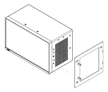
3. On the second MPS, use a Phillips-head screwdriver and 2 flat-head screws (M4 X 8) to connect the middle bracket to the *opposite* side of the MPS from the first.
