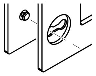
**3.** Adjust the two MPS so the holes at the back of the middle brackets are aligned.
