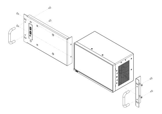
WARNING: To prevent injury or damage to the instrument, do not carry the PRISM monitor by the handles on the front of the instrument. These handles are for pulling the instrument out of a rack installation and are not intended to carry the instrument.
