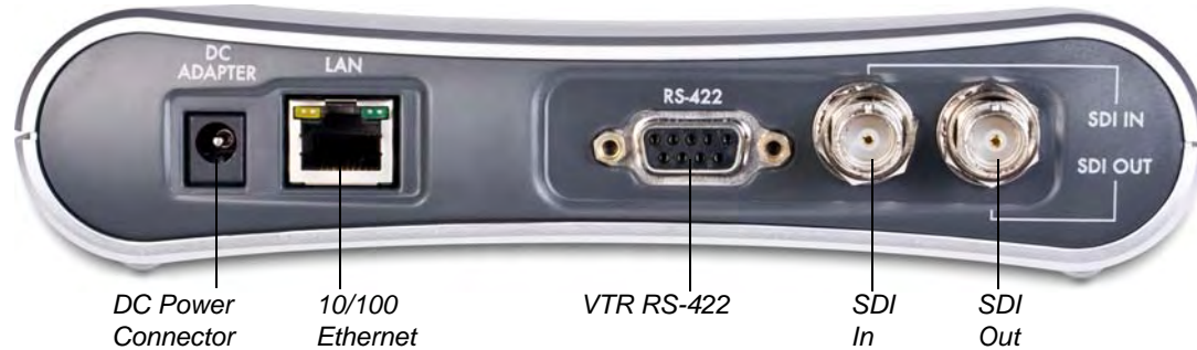
Figure 2–2. Pipeline SC rear panel
