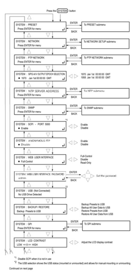
Figure 99: SYSTEM button menu diagram – part 1
