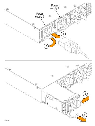
Figure 7: Removing a Power Supply module
