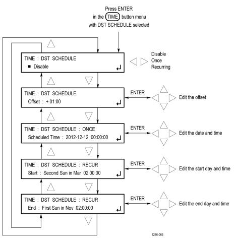
Figure 119: DST SCHEDULE submenu diagram
