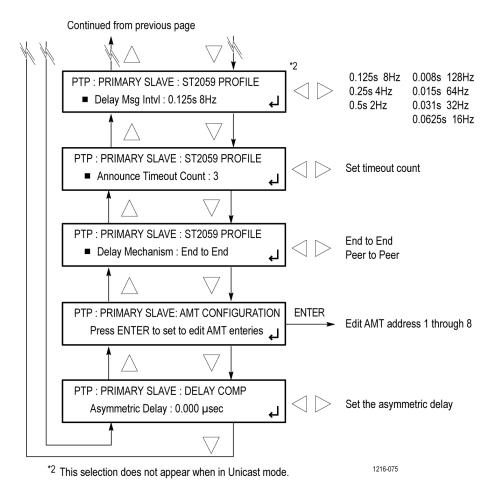
Figure 126: PTP primary slave menu diagram – part 2
