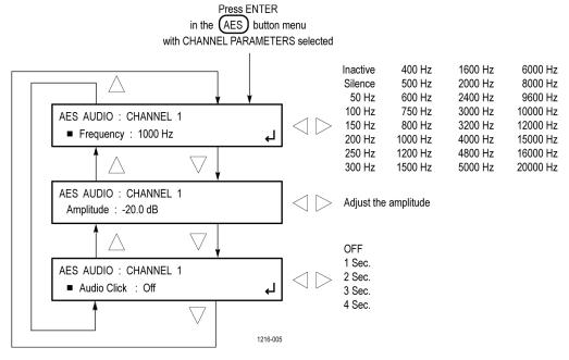
Figure 62: AES AUDIO CHANNEL submenu diagram (Option AG only)
