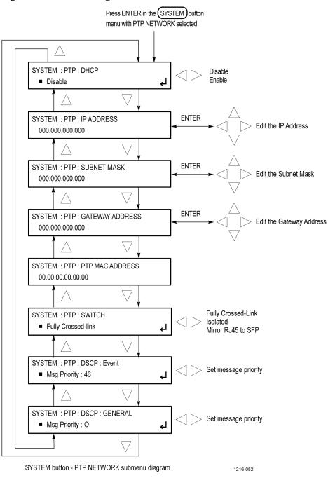
Figure 104: PTP submenu
