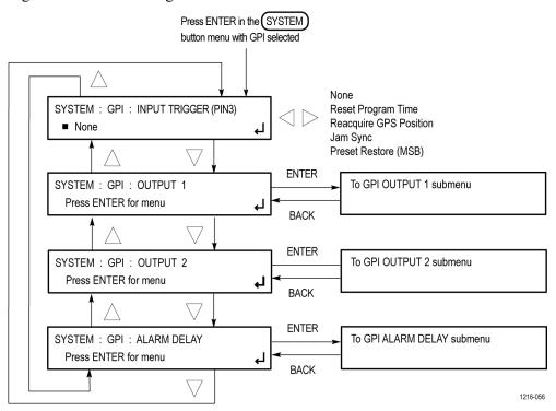
Figure 108: GPI submenu diagram
