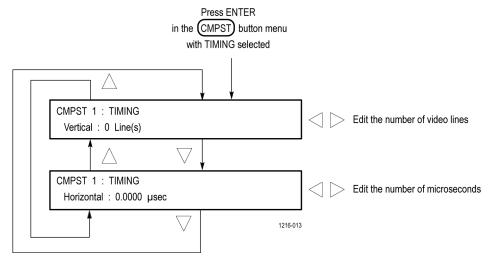
Figure 70: COMPOSITE TIMING submenu diagram
