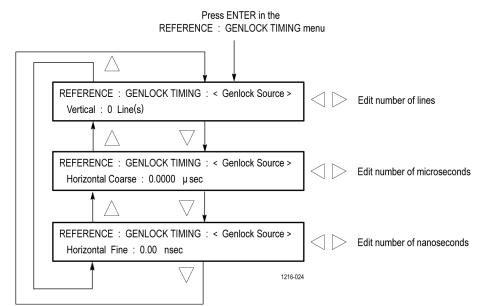
Figure 82: GENLOCK TIMING submenu diagram
