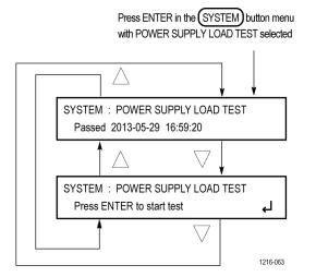
Figure 116: POWER SUPPLY LOAD TEST submenu diagram
