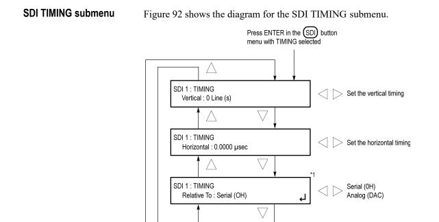
Figure 92: SDI TIMING submenu diagram
