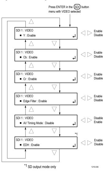
Figure 94: SDI VIDEO submenu diagram
