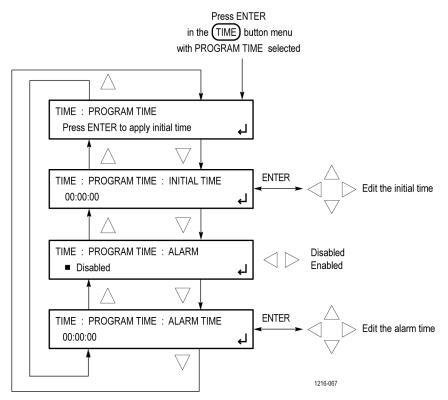
Figure 120: PROGRAM TIME submenu diagram
