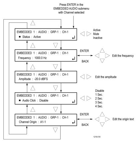
Figure 75: EMBEDDED CHANNEL submenu diagram
