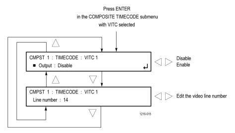
Figure 72: COMPOSITE TIMECODE VITC submenu diagram
