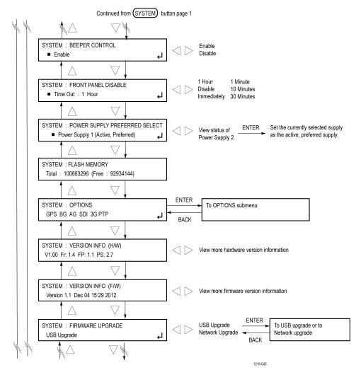
Figure 100: SYSTEM button menu diagram - part 2
