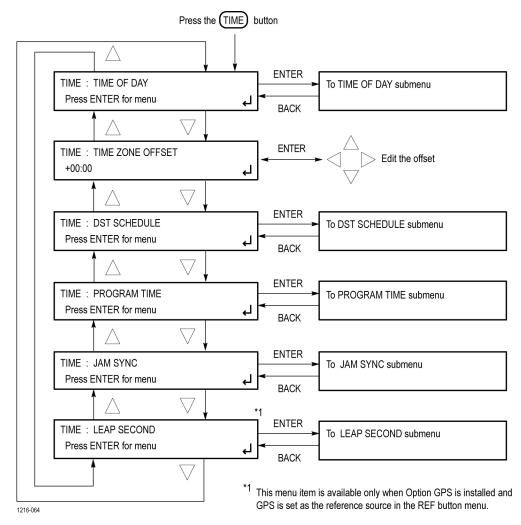
Figure 117: TIME button menu diagram
