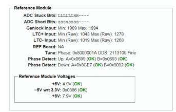
Figure 49: Reference Module diagnostic readouts
