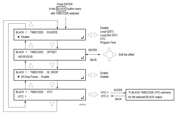
Figure 67: BLACK TIMECODE submenu diagram
