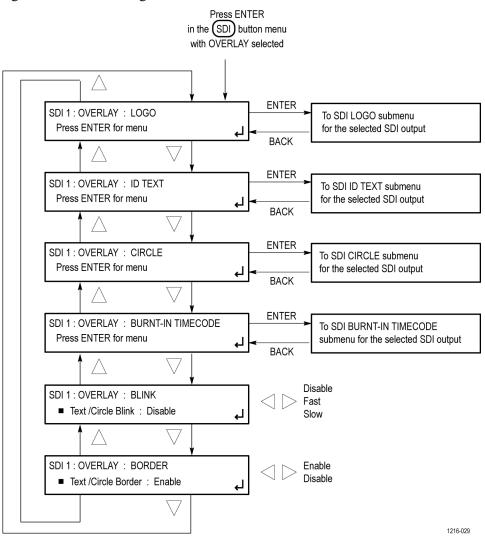
Figure 87: SDI OVERLAY submenu diagram
