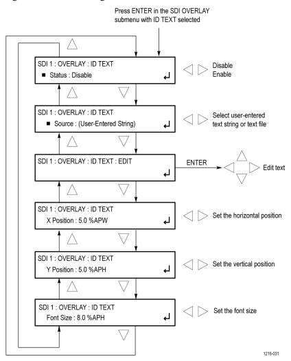
Figure 89: SDI OVERLAY ID TEXT submenu
