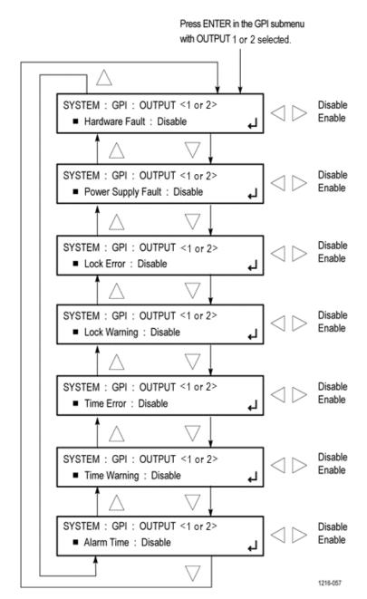
Figure 109 shows the diagram for the selected GPI OUTPUT submenu <1 or 2>.
