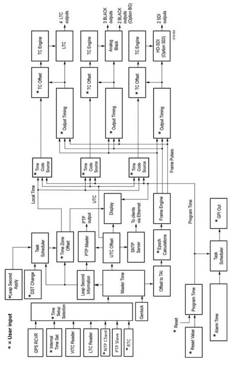
Figure 1: Time flow block diagram
