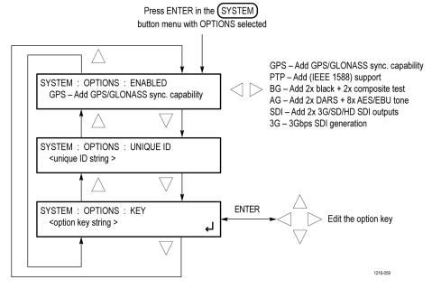
Figure 111: OPTIONS submenu diagram
