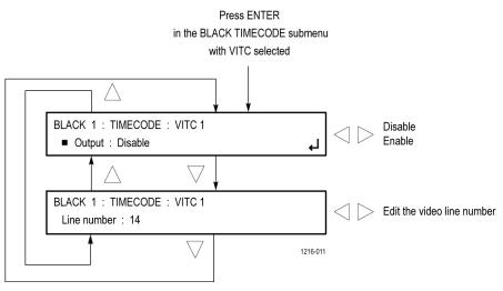
Figure 68: BLACK TIMECODE VITC submenu diagram
