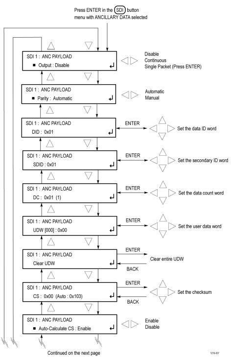
Figure 95: SDI ANC PAYLOAD submenu diagram – part 1
