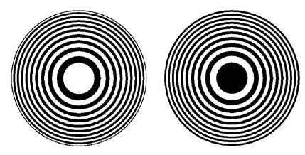
Figure 31: Optical zone plates (enlarged)
