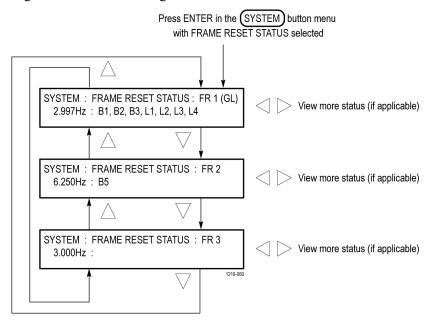
Figure 112: FRAME RESET STATUS submenu diagram
