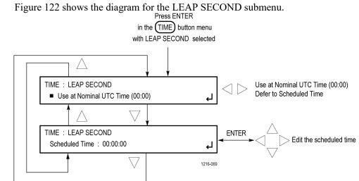
Figure 122: LEAP SECOND submenu diagram
