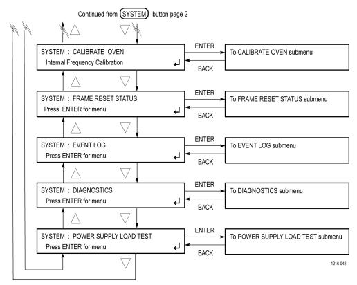
Figure 101: SYSTEM button menu diagram – part 3
