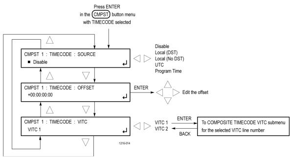
Figure 71: COMPOSITE TIMECODE submenu diagram
