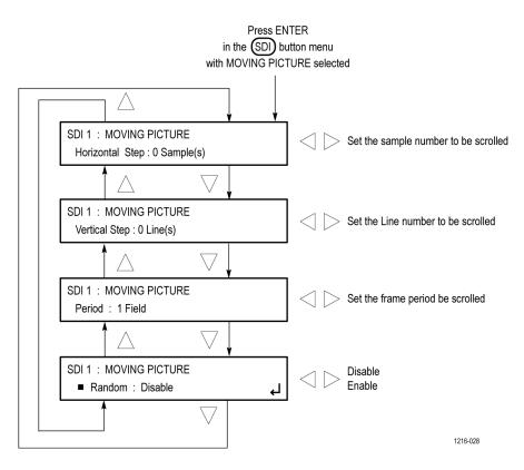
Figure 86: SDI MOVING PICTURE submenu diagram
