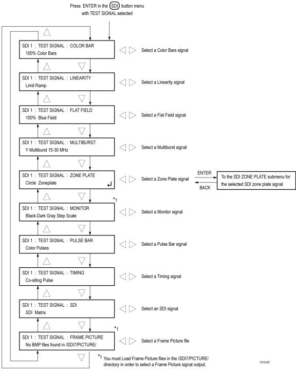
Figure 85: SDI TEST SIGNAL submenu diagram
