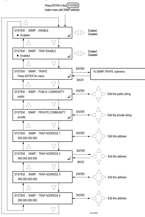
Figure 105: SNMP submenu diagram
