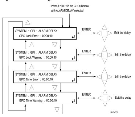
Figure 110: GPI ALARM DELAY submenu diagram
