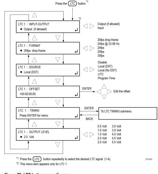
Figure 78: LTC button menu diagram
