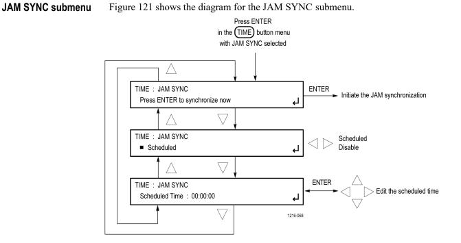
Figure 121: JAM SYNC submenu diagram
