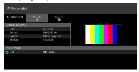
Figure 175: IP Generator application – VIDEO tab display
