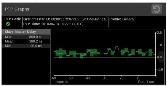
Figure 159: PTP Master-Slave Delay and Variation graphs
