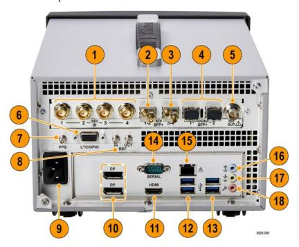
Figure 10: PRISM MPI2-10 rear panel
