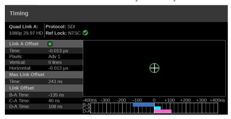
Figure 125: Timing application display for Quad Link SDI signals
