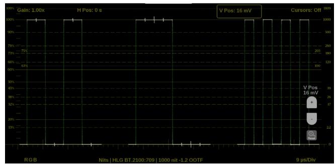
Figure 87: Waveform on-screen tools – vertical position
