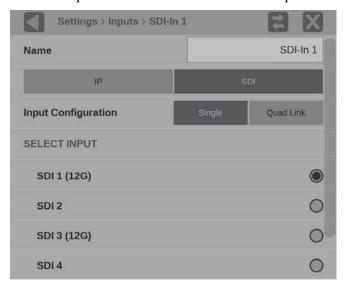
Figure 29: Single SDI signal configuration
