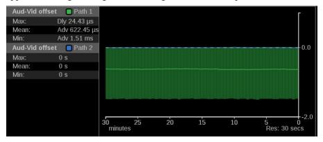
Figure 165: Stream Timing application – Audio to Video graph
