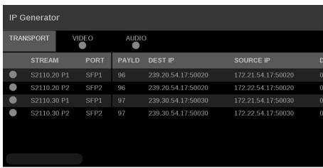
Figure 174: IP Generator application – TRANSPORT tab display
