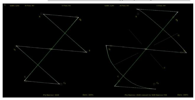
Figure 45: Vector display with (right) and without (left) Convert to Rec. 709 enabled, 100% color bar in PQ/BT.2020
