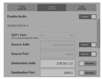
Figure 38: Enabling a ST2110-30 audio stream
