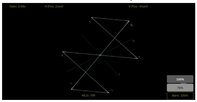
Figure 99: Vector on-screen tools – Bar Targets
