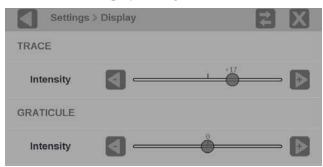
Figure 69: Trace and graticule intensity sliders
