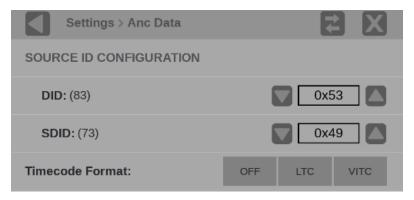
Figure 56: Reference configuration Anc Data
