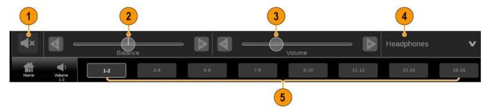
Figure 75: Mute, balance, volume, device, and source controls
