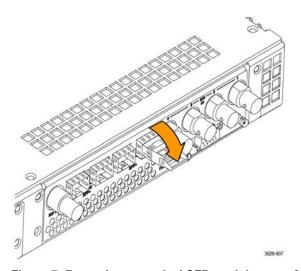
Figure 7: Removing an optical SFP module on an MPX2-10 monitor
