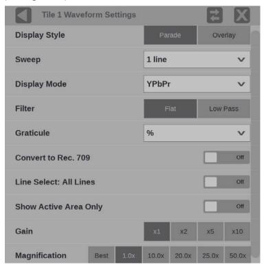
Figure 83: Waveform application settings menu
