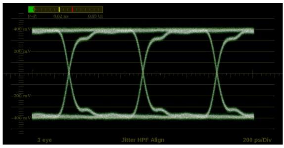
Figure 186: Eye Display application display
