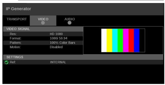
Figure 169: IP Generator application display
