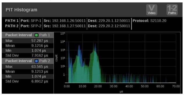
Figure 153: PIT Histogram application display
