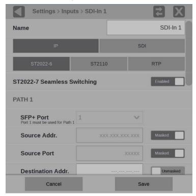
Figure 35: IP input protocols and ST2022-7 seamless switching
