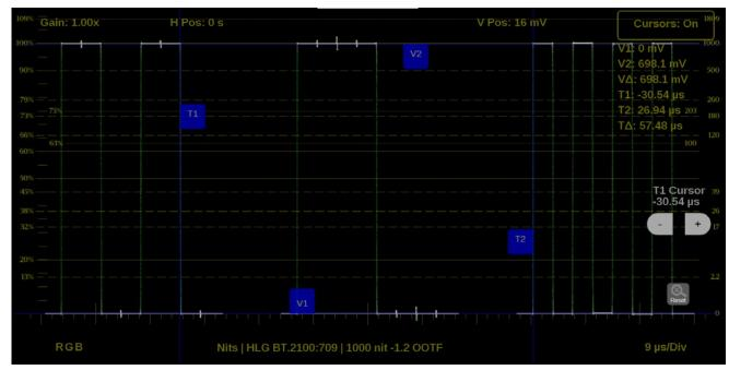
Figure 88: Waveform on-screen tools – time and voltage cursor values and deltas
