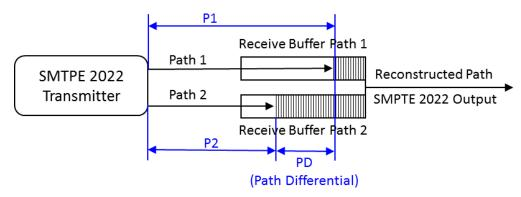
Figure 150: Seamless protection switching of SMPTE ST-2022-7 IP stream
