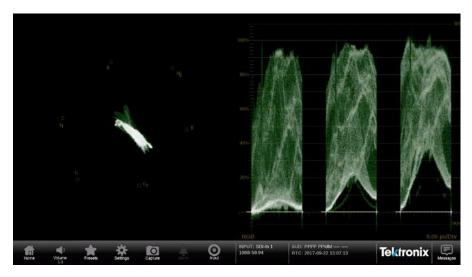
Figure 19: Two half screen tiles showing vector and waveform displays
