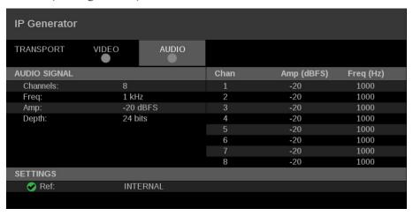
Figure 176: IP Generator application – AUDIO tab display
