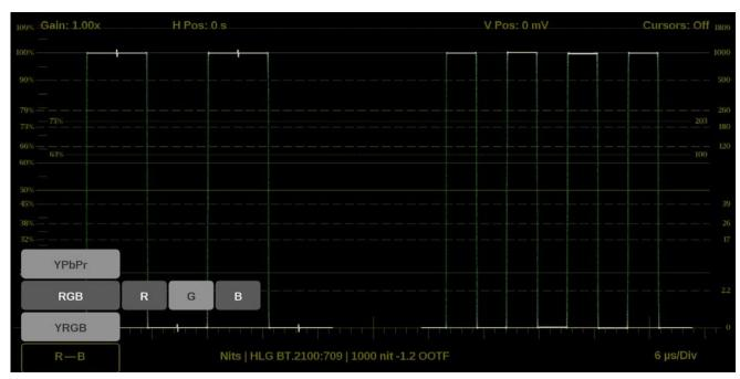
Figure 89: Waveform on-screen tools – Display Mode
