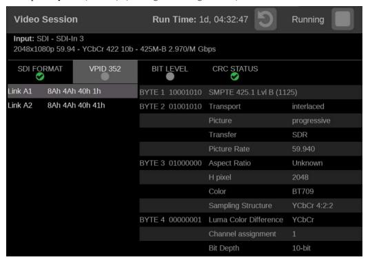
Figure 119: Video Session application — VPID 352 tab display for 3G-SDI Level B signal
