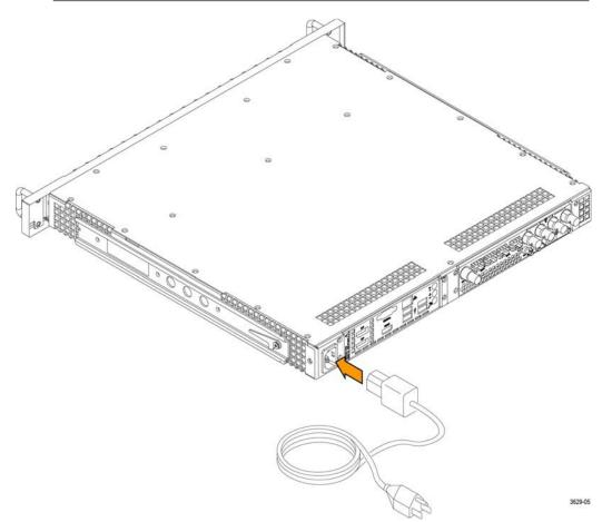
Figure 4: Connecting power to the MPX2-10 monitor
