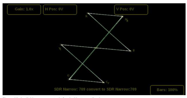
Figure 95: Available on-screen tools for the Vector application
