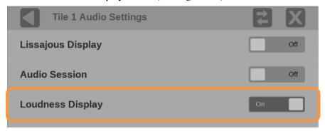
Figure 47: Audio Settings with the Loudness Display enabled
