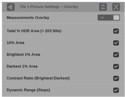
Figure 111: Picture Settings with Measurement Overlay menu
