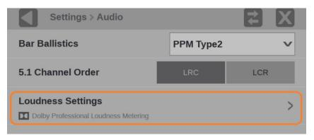
Figure 49: Audio submenu with the Loudness Settings marked
