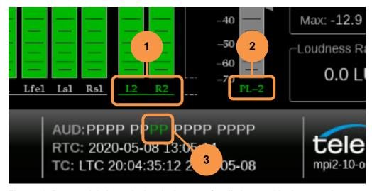
Figure 52: Program labels marked at the bottom of audio bars and in the status bar
