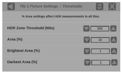
Figure 112: Picture Settings with Measurement Threshold menu
