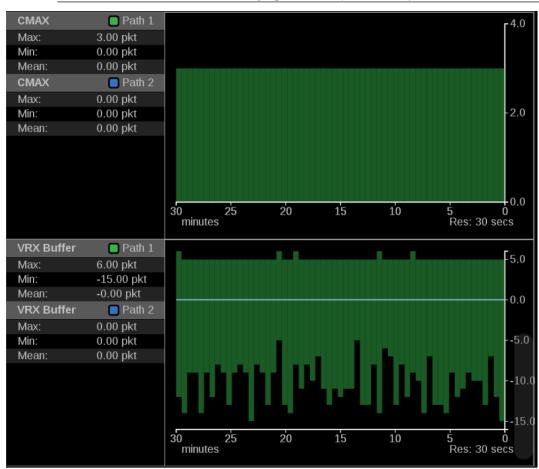
Figure 152: IP Graphs application - CMAX and VRX Buffer graph
