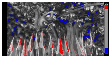
Figure 115: Luminance False Color display with Meter Overlay
