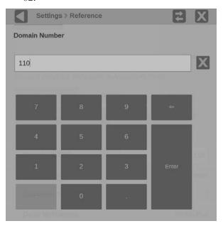
Figure 62: Domain number keypad for the PTP domain setting
