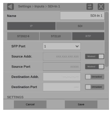
Figure 40: Configure RTP
