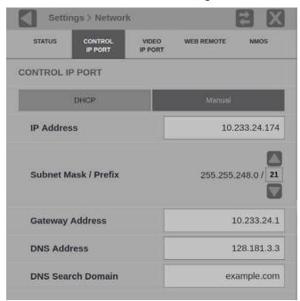
Figure 9: Setting network parameters
