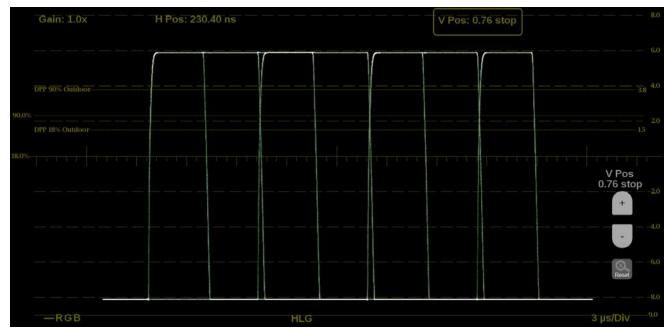
Figure 195: Stop Display on-screen tools – vertical position
