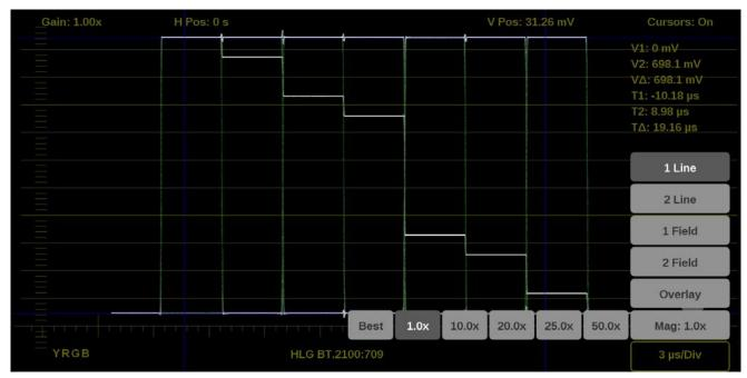
Figure 90: Waveform on-screen tools – display format
