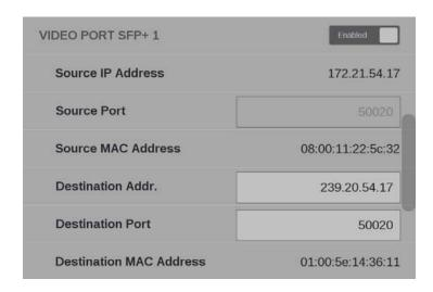
Figure 172: Video Port SFP configuration
