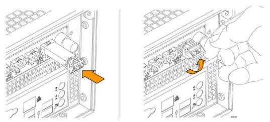
Figure 6: Installing and removing an optical SFP module on an MPI2-10 monitor
