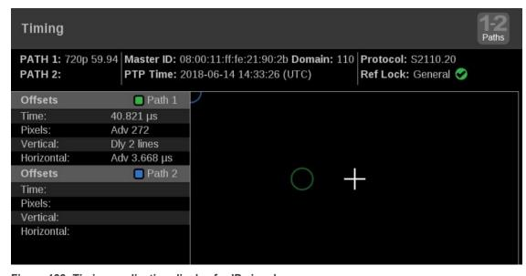
Figure 122: Timing application display for IP signals
