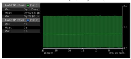
Figure 166: Stream Timing application – Audio to RTP graph
