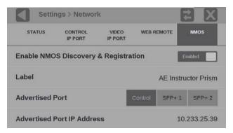
Figure 46: NMOS discovery and registration enabled
