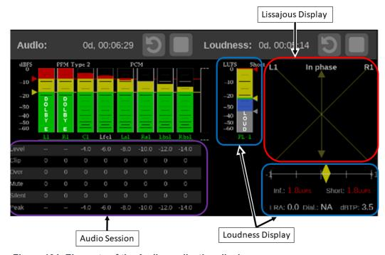
Figure 104: Elements of the Audio application display
