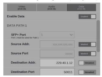
Figure 39: ST2110-40 data stream enabled
