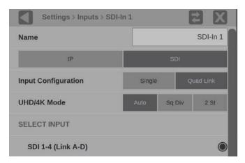
Figure 30: Quad Link SDI signal configuration
