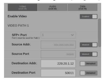
Figure 37: Enabling a ST2110-20 video stream
