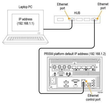
Figure 8: Connecting the instrument to a PC (MPI2-10 monitor shown)
