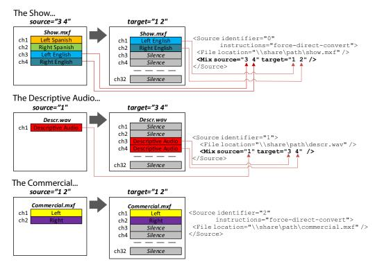
From *Source* 0 (the show itself), the *Mix* element specifies that only channels 3 and 4 should be utilized—as channel 1 and 2 in the output—in any *Segment* where this *Source* is used.
