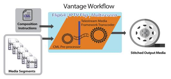
In transcode workflows, uncompressed baseband video is presented; in direct-convert mode, original compressed frames are presented. The media segments in the CML must be of the same resolution—same frame size (width and height)— and frame rate. Audio is always presented as uncompressed PCM.
