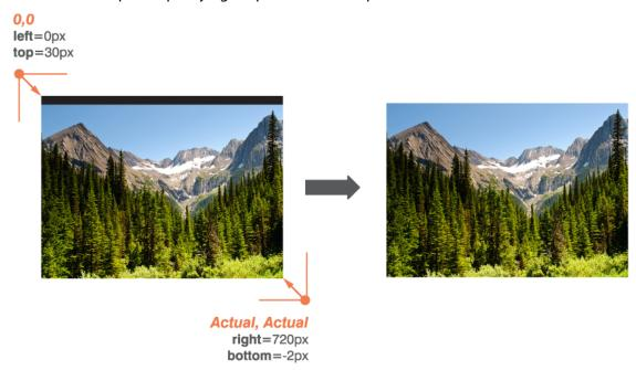
In this example, VBI is being stripped from SD source using pixels: 30 pixels from the top, 2 pixels from the bottom.
