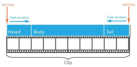
By definition, a Head can not begin (have a time) before the beginning of the instance. It can be later (with an Edit), and it can have an effect duration (Fade), extending to the right (forward) along the instance. Similarly, a Tail can not be later than the end of the instance, but it can be earlier with an Edit, and it can also have a Fade, extending in this instance backward along the instance.
