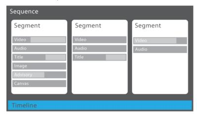
Also recall that each sequence creates an independently-functioning timeline within a composition—the point of a sequence is to provide you a new, independent timeline upon which you can place segments of material and play them independently of any other material in the composition.
