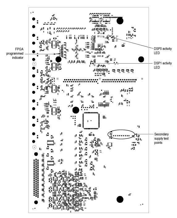
Figure 5: Options AD and DPE Audio board back side indicator LED and test point locations
