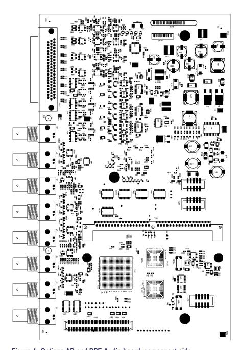
Figure 4: Options AD and DPE Audio board, component side
