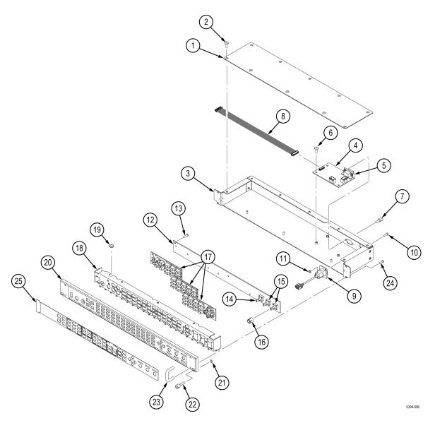
Figure 9: Replaceable parts (WVR8RFP Remote Front Panel)
