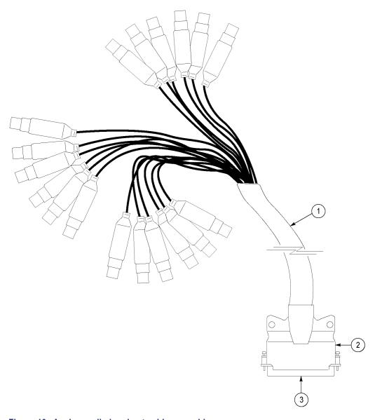
Figure 10: Analog audio breakout cable assembly
