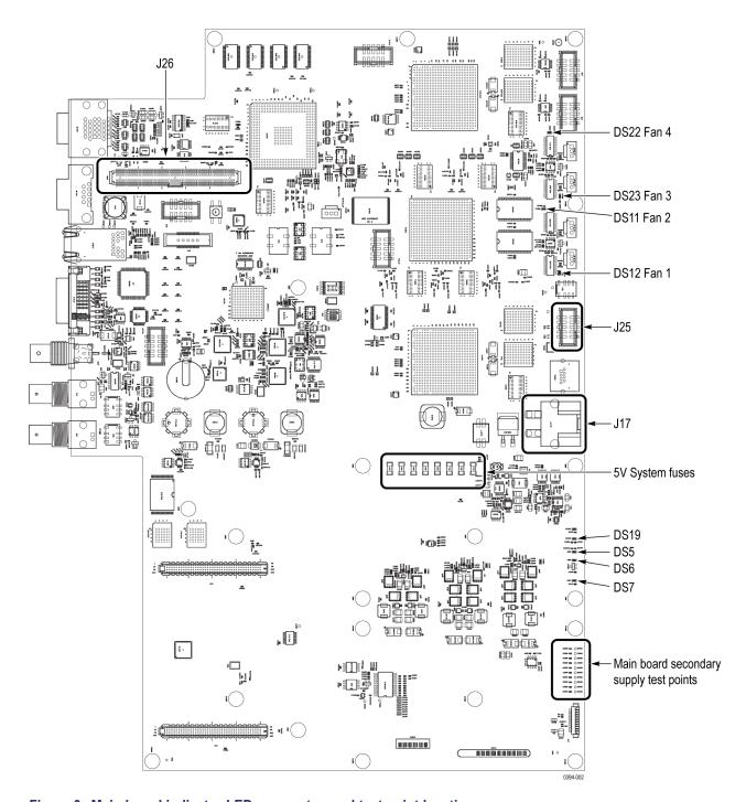
Figure 3: Main board indicator LED, connector, and test point locations
