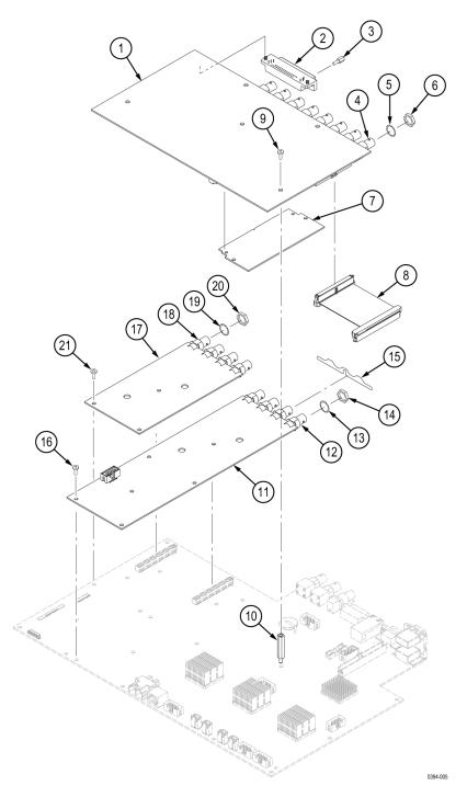
Figure 8: Replaceable parts (options)
