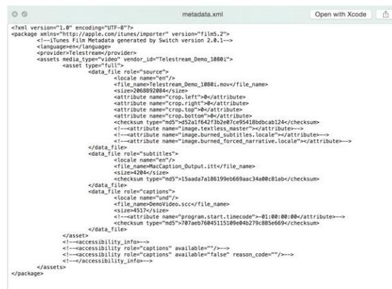
**Figure 7. Example of XML file generated from Switch ITMP export**
