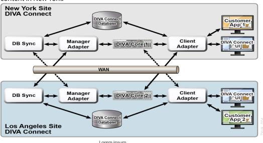
Though it is technically possible to configure Customer App 2 to remotely connect to New York's ClientAdapter, this configuration often provides better availability, security, and auditing. Performance and scalability is often increased as well, especially with
